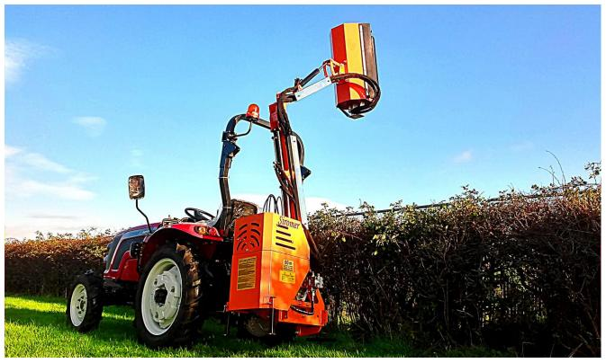
Siromer Hedge Trimmers are designed to fit industry standard CAT I linkages. Siromer's high reach hedge trimmers are fitted with a PTO driven hydraulic pump, which means the hedge trimmer is independent of the tractor's hydraulics. The finger bar and flail heads are interchangeable. See price list for costs.
