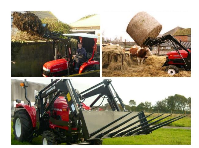
The Siromer Loaders can be fitted with a fork attachment. The fork attachment comes complete with 7 tines 1m in length. They are fitted with euro brackets to attach to the Siromer Loaders.
